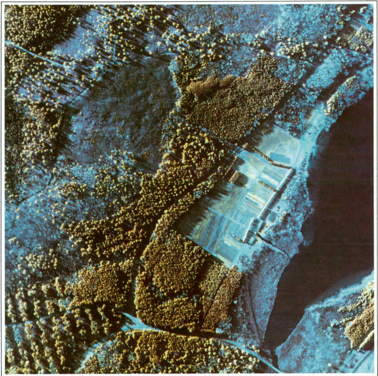
Digital image of the Petawawa Forest Research Institute acquired by the CCRS solid state Multispectral Electro-optical Imaging Scanner (MEIS) from 1750 m. Pixel size is 1.2 m by 1.2 m. Pixels (for 'picture elements') are the smallest constituents of an image. This type of digital imagery can be used for forest regeneration and inventory work.
