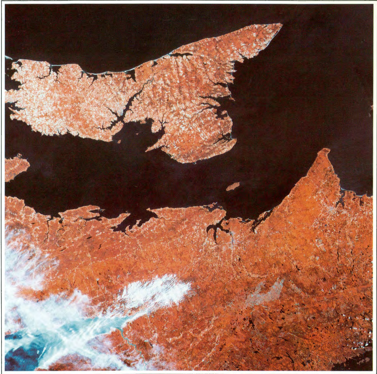
LANDSAT MSS image with nominal 80 m resolution, from July 3, 1981, covering an area of 185 km by 185 km, including much of Prince Edward Island. This type of image can be used to study cropland distribution, general land use and regional geography.
