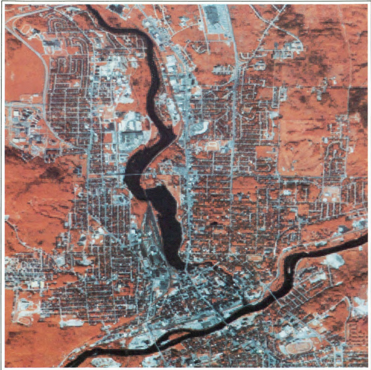
SPOT simulation of Sherbrooke, Quebec, which integrates the 10 m resolution panchromatic band and the 20 m multispectral data. This image was produced from airborne digital multispectral scanner data acquired by CCRS in November 1982. It is expected that topographic map revision and detailed land cover mapping will be significant applications of SPOT data. Photo courtesy of Sherbrooke University.
