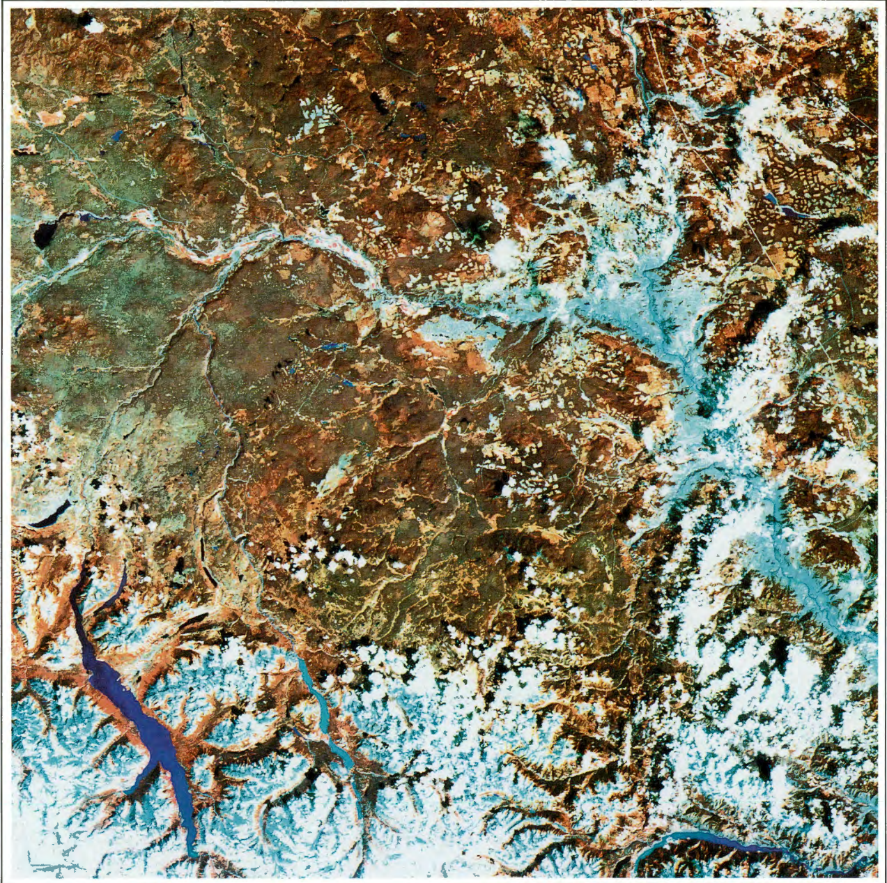
A LANDSAT MSS softwood enhancement of part of the Cariboo plateau region of interior British Columbia. The Fraser River flows south along the eastern edge. Lodgepole pine stands appear dark green, with varying amounts of red depending on deciduous vegetation present. The imagery can be used for cutover mapping (small, often rectangular yellow-orange areas) and general forest inventory.
