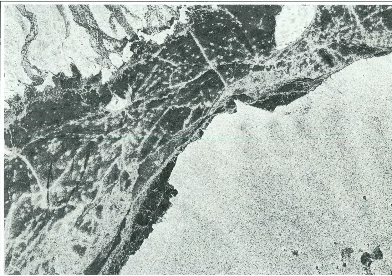
Synthetic aperture radar image from the SEASAT mission, July 1978, showing a portion of Banks Island, NWT, in the top left corner. Smooth, shore-bound ice along the coastline reflects the microwaves emitted by the radar away from the sensor, and therefore appears dark. Open water, because it is rippled, reflects part of the incident energy towards the radar, and therefore appears grey. Such imagery is used in studies of ice as well as for navigation. Digital Processing: MacDonald, Dettwiler & Associates Ltd.
