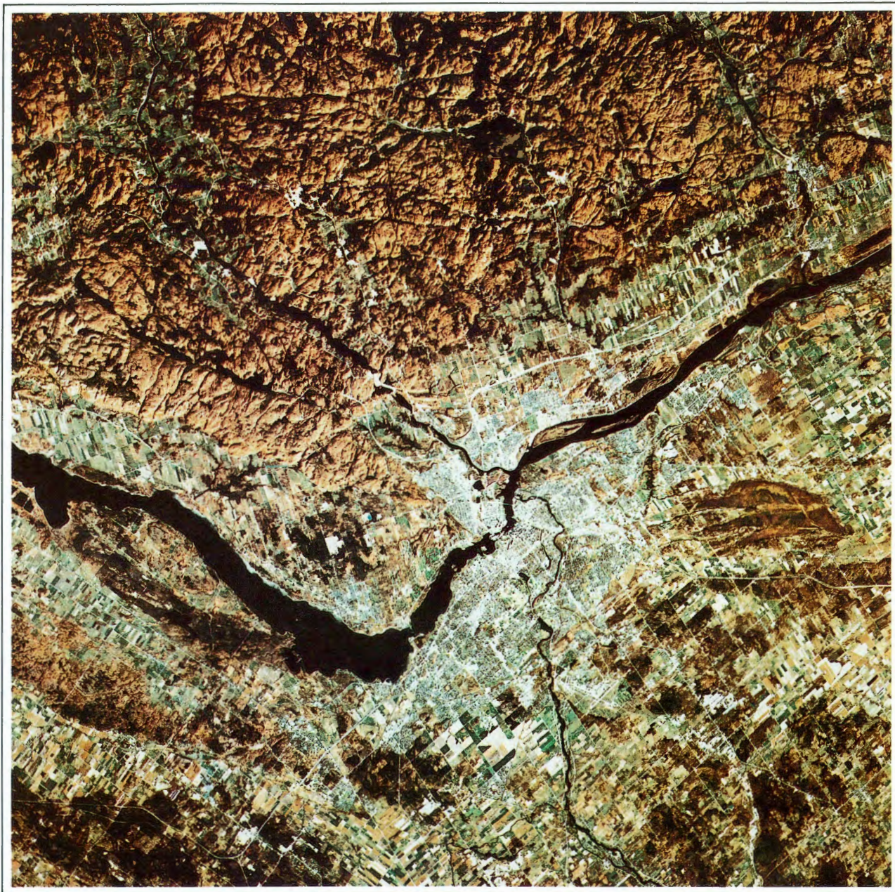
The first 30 m resolution LANDSAT-5 Thematic Mapper image of Ottawa. On photographic print, individual subdivision roads and larger buildings are clearly discernible. This type of image can be used for land use, land cover, forestry, wildlife habitat and related mapping and monitoring applications.
