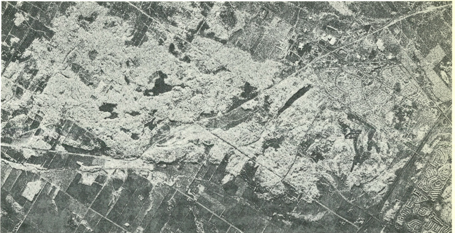
C-band synthetic aperture radar image of Kanata, Ontario showing urban, agricultural and forested land.
