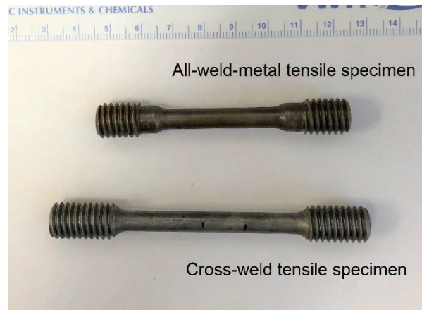
Figure 3. Etched AWM and cross-weld tensile specimens of TC128B longitudinal weld.
