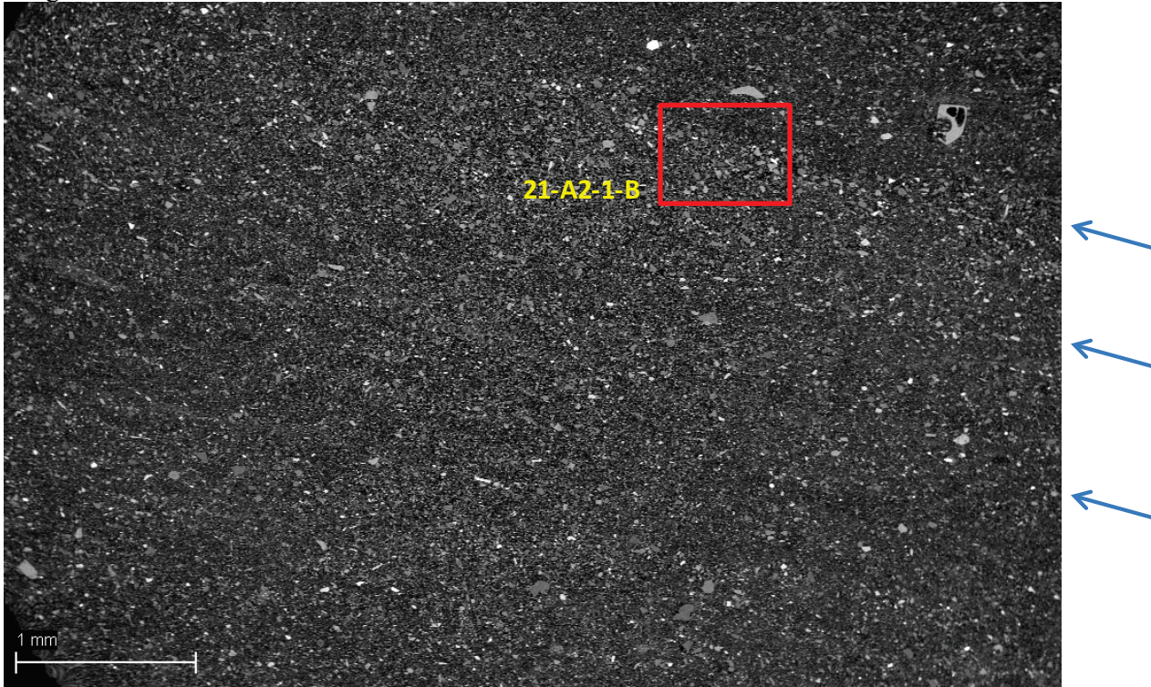
Figure A-32. BSE micrograph showing interstratified coarse (light) and fine (dark) sub-horizontal laminae. The contacts between the coarse and fine laminae are diffuse and generally indicated by arrows.
