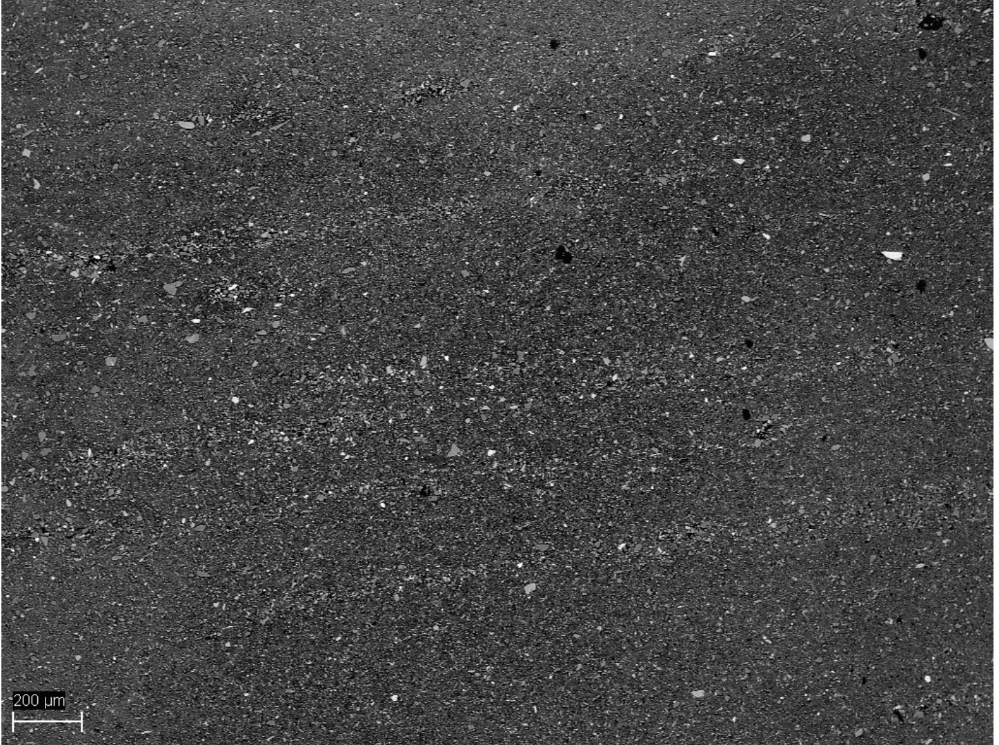
Figure A-1. Backscattered electron (BSE) micrograph showing sub-horizontal laminae in the silt- and clay-size fraction with few grains of very fine to fine sand-size. Coarse laminae are laterally discontinuous and are of variable thickness with poorly-sorted angular to sub-angular, matrix-supported clasts. The presence of laminae suggests that grains were hydraulically sorted and segregated during sediment transport.
