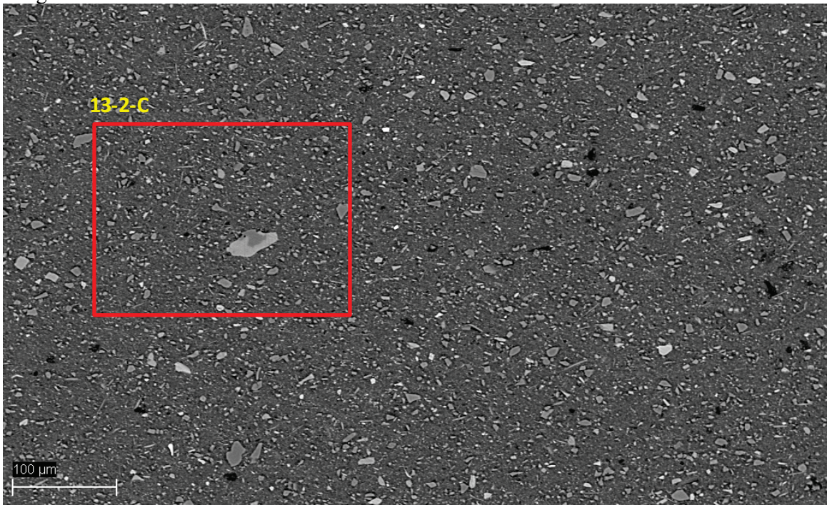
Figure A-17. BSE micrograph showing massive texture of sediment, with an absence of laminae or lenses. Grain size ranges from coarse silt (50 µm) to clay ( \leq 2 µm).
