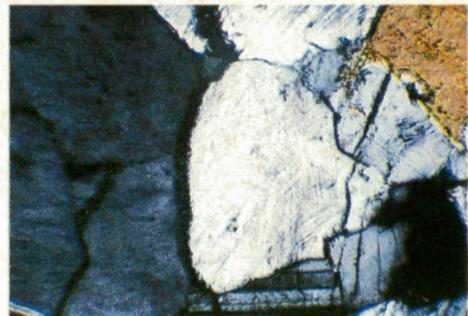
*Figure 1b Photomicrograph of shock-induced planar features in quartz (light grey) from the Mistastin impact structure, Labrador*
