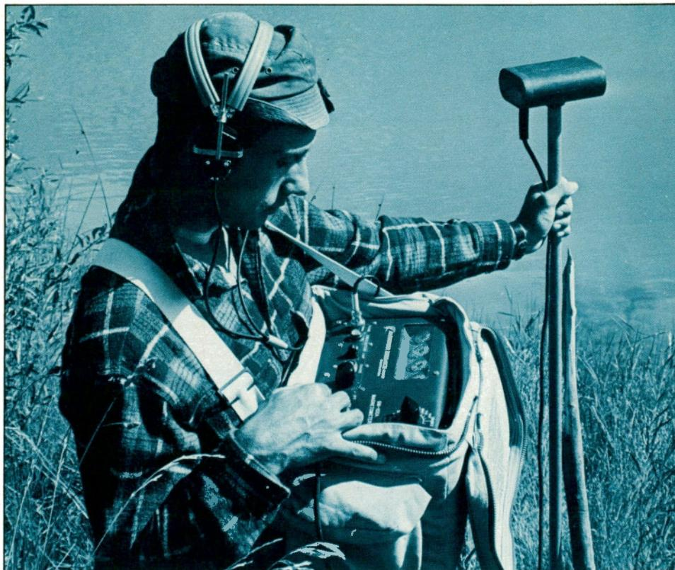
The Barringer GM-102 proton precession magnetometer, the first commercial portable ground prospecting instrument to utilize the Serson patent for a direct digital readout of the total intensity of the earth's magnetic field. Dr. P. Serson, a former EMR scientist holds the patent.
