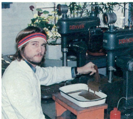
Research technician Geoffrey Leigh performing the flotation process on gold tailing ore. The brown froth coming out of the flotation cell contains gold concentrate.
