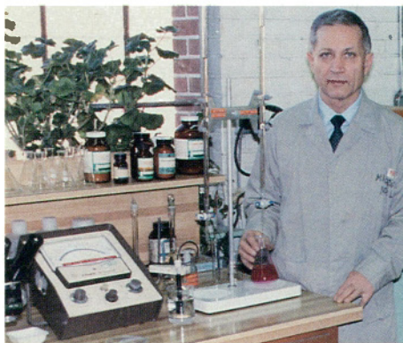
Research scientist Marius Cristovici monitors and adjusts the cyanide and lime (pink bottle) concentration in solution by titration. The second step in the CANMET process is called cyanidation.
