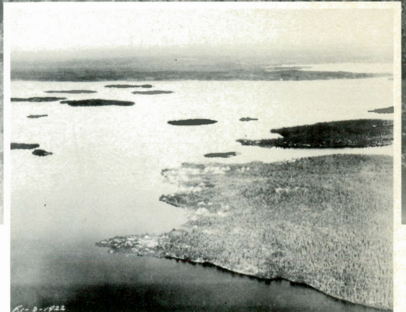
The 1922 aerial photo of Pelican Narrows taken with an Eastman K-2 camera with a 30 cm focal length. Altitude 914.4 m.
