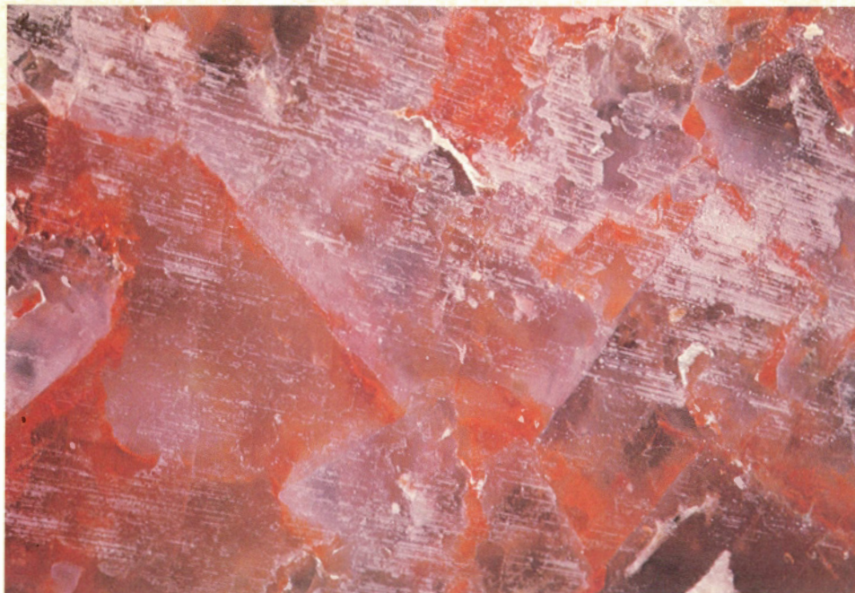
Figure 1 Potash ore darkens with iron oxides and water-insoluble clays
