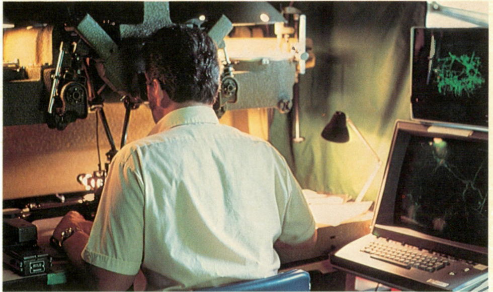
Photogrammetric Digital Data Acquisition System. Television-like terminals display digitized terrain features extracted by the technician from a pair of aerial photographs viewed through binoculars of the B-8 stereoplotter
