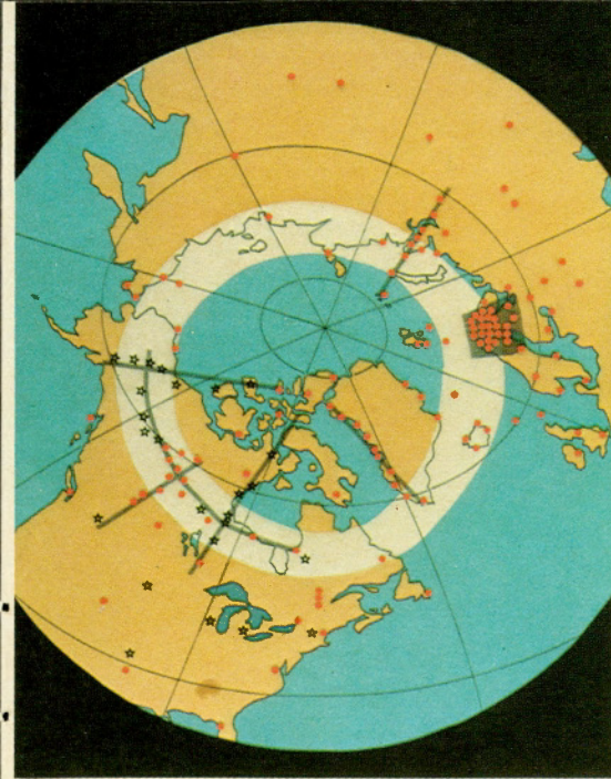
Figure 4. The auroral zone and the distribution of IMS magnetic stations. Stars are stations with real-time telemetry facilities
