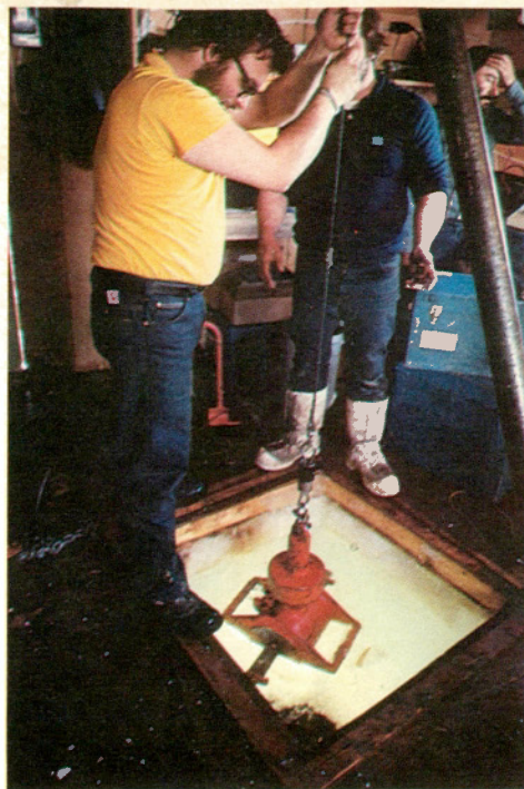
Stephen Blasco, Geological Survey of Canada, lowers a grab sampler through a hole in the ice platform
