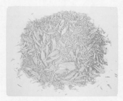
Fig. 2. The cast bar of commercially pure tin shown in Fig. 1 after inoculation with gray tin and 13 days at -30 °C.
