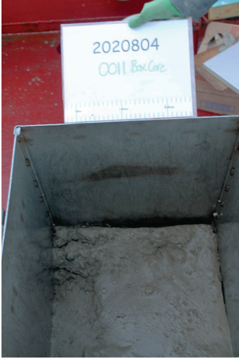
D 1. Deck photo of Van Veen grab contents at station 0011. Photograph by V. Kostylev. NRCan photo 2020-605.
