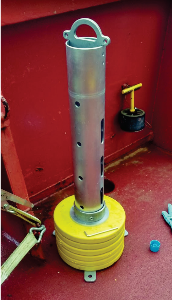
Figure 6. The new GSC(A) MK 3 gravity core head. Photograph by V. Kostylev. NRCan photo 2020-598.
