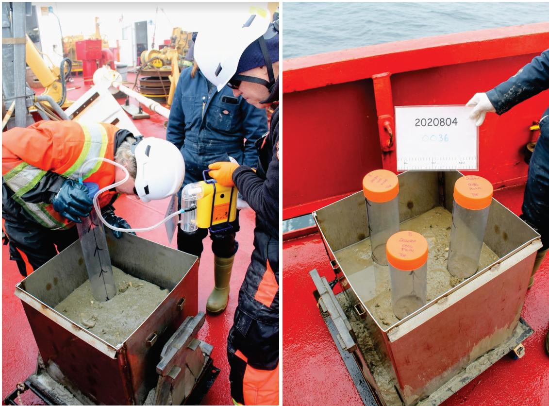
Figure 7. Use of vacuum pump for obtaining push cores on board Amundsen 2020804. Photographs by V. Kostylev. NRCan photos 2020-599, 2020 – 600.
