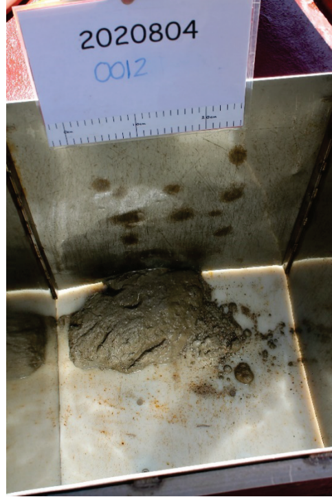
D 2. Deck photo of box core contents at station 0012. Photograph by V. Kostylev. NRCan photo 2020-606.
