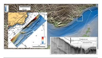
**Figure 21.** Seabed mapping based on multi-beam bathymetry, backscatter and sub-bottom geophysics.
