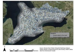
Figure 4: Fine FEM incorporating Strahler Order 3+ streams from the Ontario Integrated Hydrology Dataset. The FEM contains approximately 133,000 nodes per sheet.
