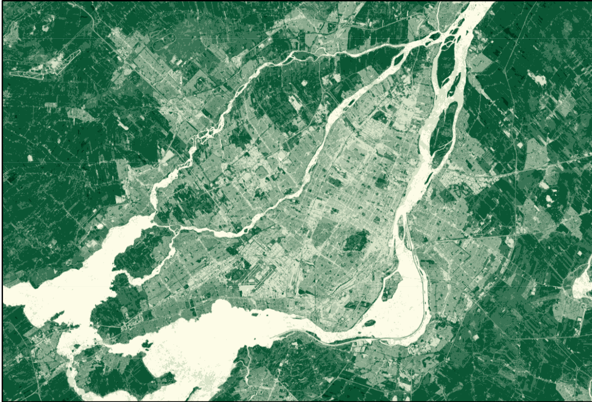
Figure 13.1 – A Normalized Difference Vegetation Index (NDVI) map dynamically generated from the 2014 landsat-8 national mosaic at 30m spatial resolution hosted inside the Data Cube Platform.
