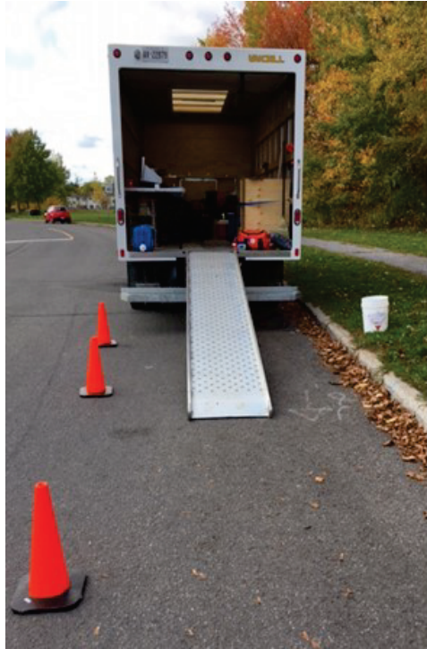
Figure A1. Rental cube truck, as a portable field lab, containing the essentials for core preservation; Photos: GSC, Oct 2019
