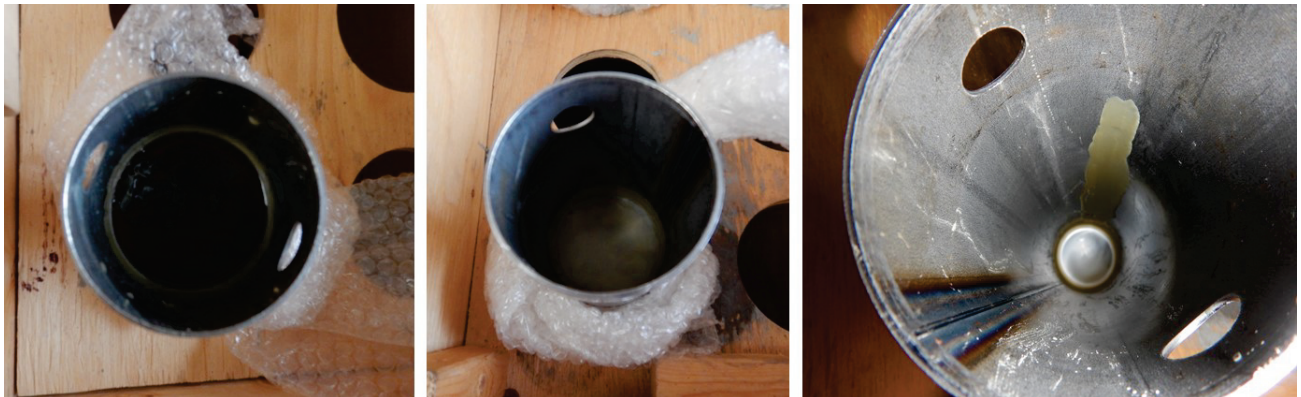
Figure 6. Gradual cooling and solidification of wax mixture on the surface of the sediments. Photos: GSC, Oct 2019
