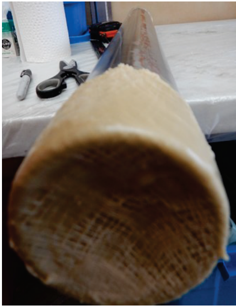
Figure 13. One layer of wax after applying the cheesecloth does not provide a uniform coating. In this example, 2-3 more dips into the wax mixture were required. The concave base of the sediment core is typical of most sediment cores in this study. Photo: GSC, Nov 2019
