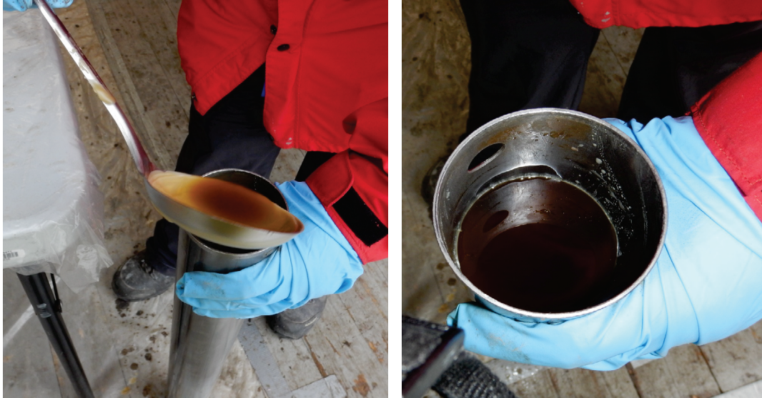
Figure 5. Ladling the molten wax mixture onto the sediment surface to preserve the sample at the top end of the Shelby tube; Photos: GSC, Oct 2019
