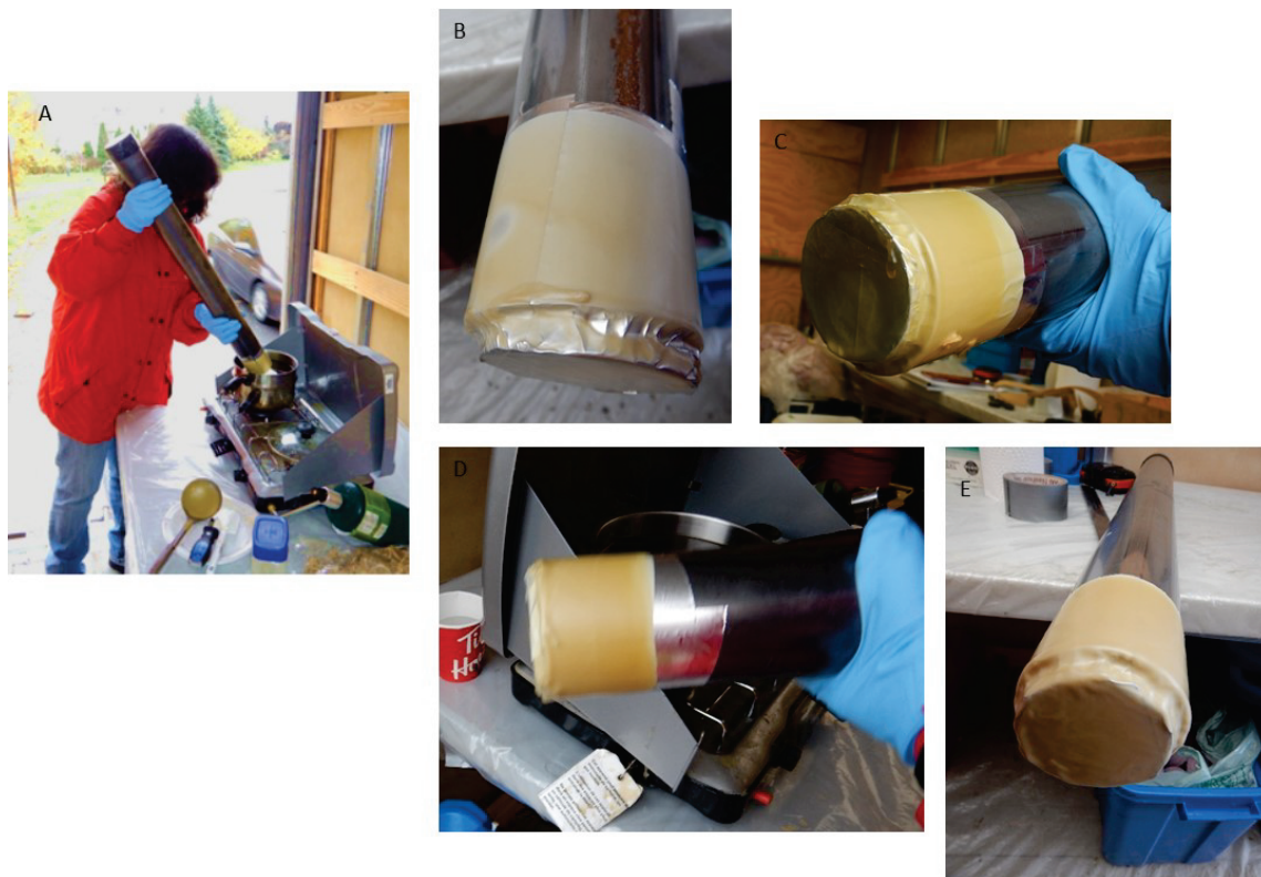
Figure 9. Adding the first wax layers on top of the aluminum foil tape (A) Gently inverting the top of the Shelby tube to dip it into the warm wax mixture. (B) The first layer of wax does not usually apply a full homogeneous coating. (C) and (D) Subsequent coatings allow for better coverage of the core end. (E) Once sealed, the thickness of the wax mixture coating is more even. Photos: GSC, Oct-Nov 2019
