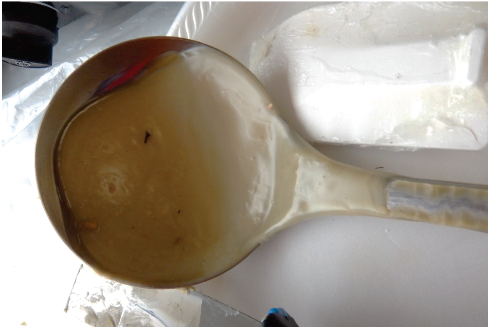
Figure 3. Impurities in the industrial grade brown beeswax (shown on a metal ladle) do not impede the effectiveness of the wax mixture as a sealant when applied in multiple layers. Photo: GSC, Oct 2019
