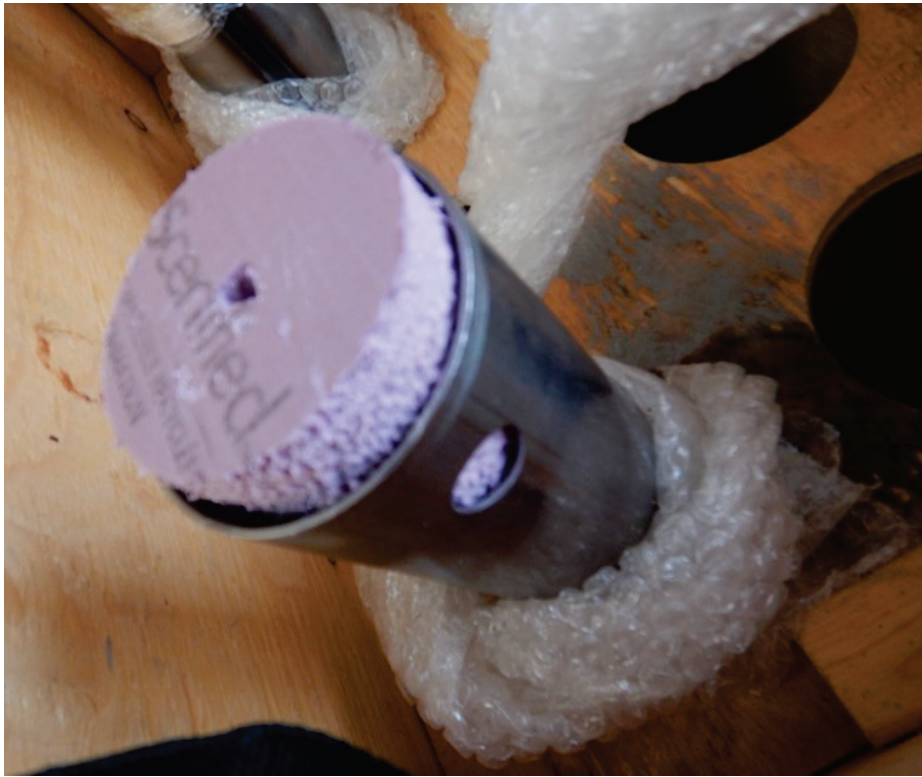
Figure 7. Rigid polystyrene insulation disks fill the void space above the surface of the sediments in the Shelby tube. In future coring, the top-most polystyrene disk will be cut to be almost flush with the top end of the Shelby tube. Photo: GSC, Oct 2019
