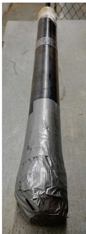
Figure 14. Additional sealing for a sediment sample that protruded beyond the bottom of the Shelby tube; Photo: GSC, Dec 2019
