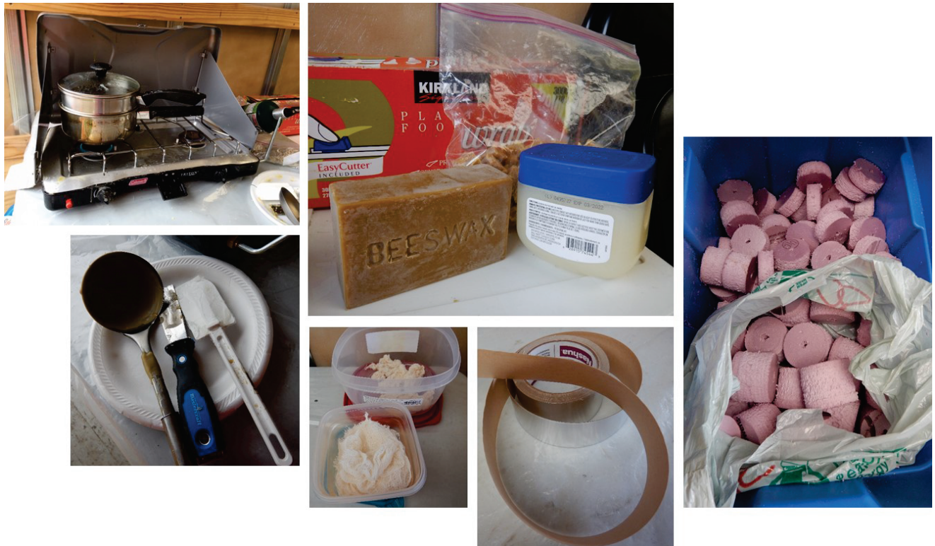
Figure A2. Supplies for wax sealant of samples in Shelby tubes, clockwise from top left: Double boiler on camp stove; Plastic food wrap, industrial-grade brown beeswax, petroleum jelly; Disks cut from rigid insulation sheets; Aluminum foil tape for duct work; Cheesecloth layers cut into squares; Implements for handling the wax mixture – metal ladle, putty knife, spatula. Photos: GSC, Oct-Nov 2019
