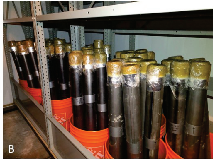
Figure 15. Transport and storage of samples. (A) The insulated shipping box became a core incubator with hot water bottles placed inside with the cores to avoid freezing when ambient field temperatures dropped. (B) For storage (several months), cores remained upright in a dedicated cold room. Photos: GSC, Nov 2019
