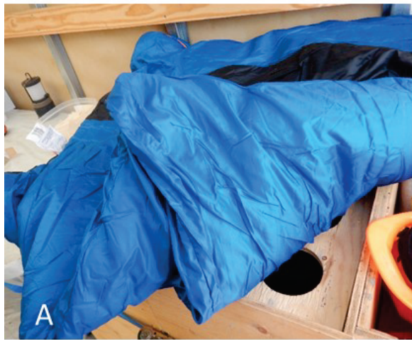
Figure 15. Transport and storage of samples. (A) The insulated shipping box became a core incubator with hot water bottles placed inside with the cores to avoid freezing when ambient field temperatures dropped. (B) For storage (several months), cores remained upright in a dedicated cold room. Photos: GSC, Nov 2019
