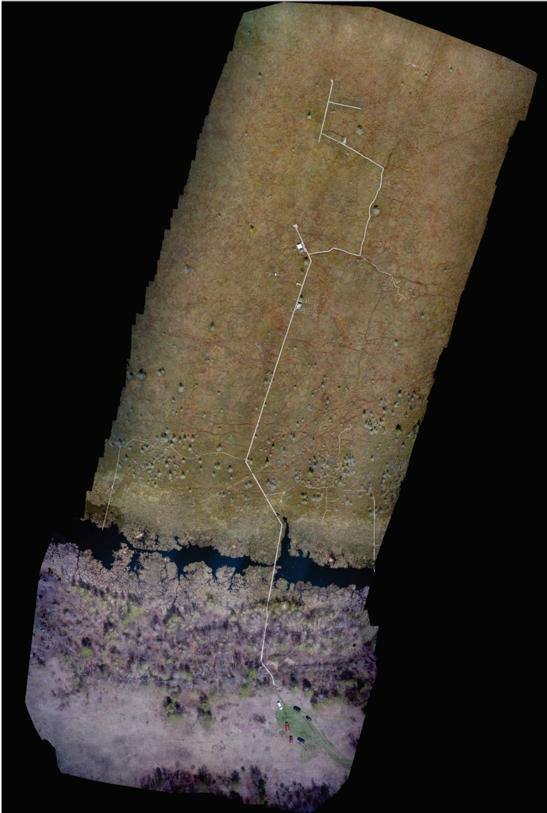
Figure 10: Orthomosaic at 1cm resolution covering part of the MBR Bog and Parking of the Parking areas based on photographs acquired with the PX8 UAV on May 12, 2016
