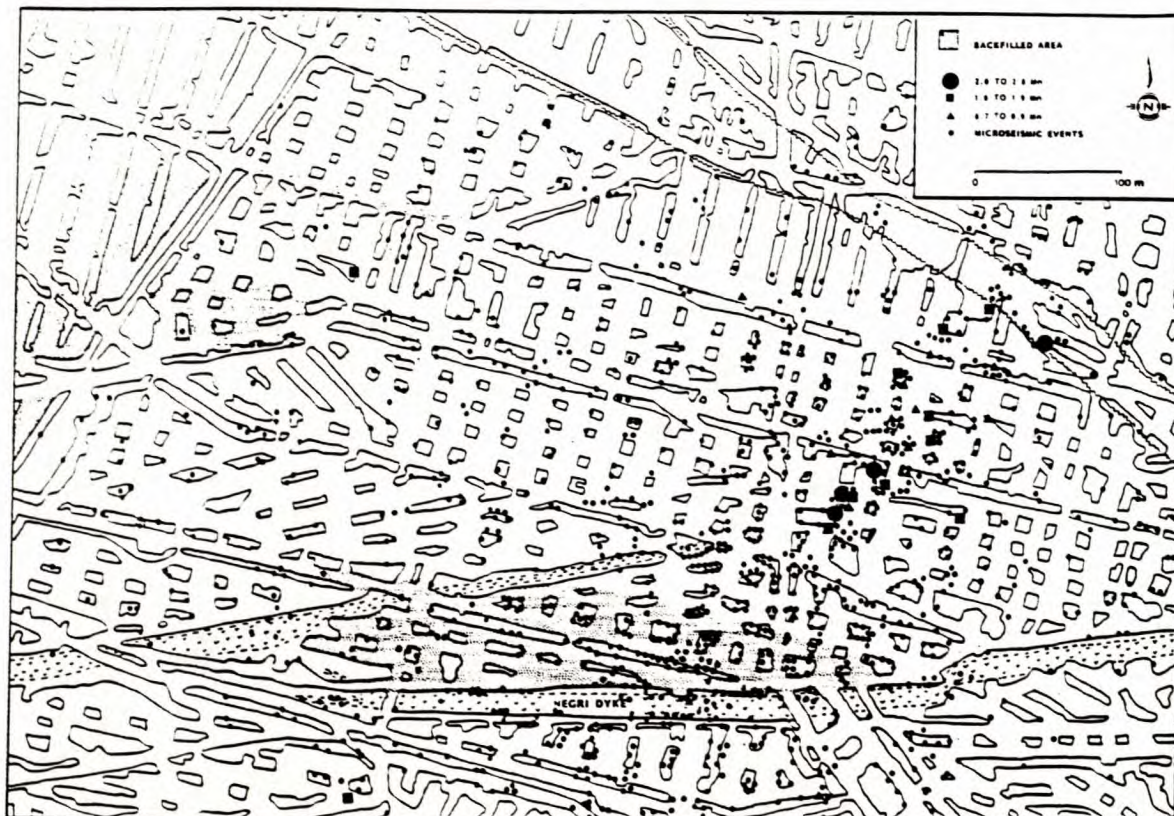
Fig. 15 - Plan of the eastern part of Denison Mine showing extent of seismic activity, 1987 to 1989.
