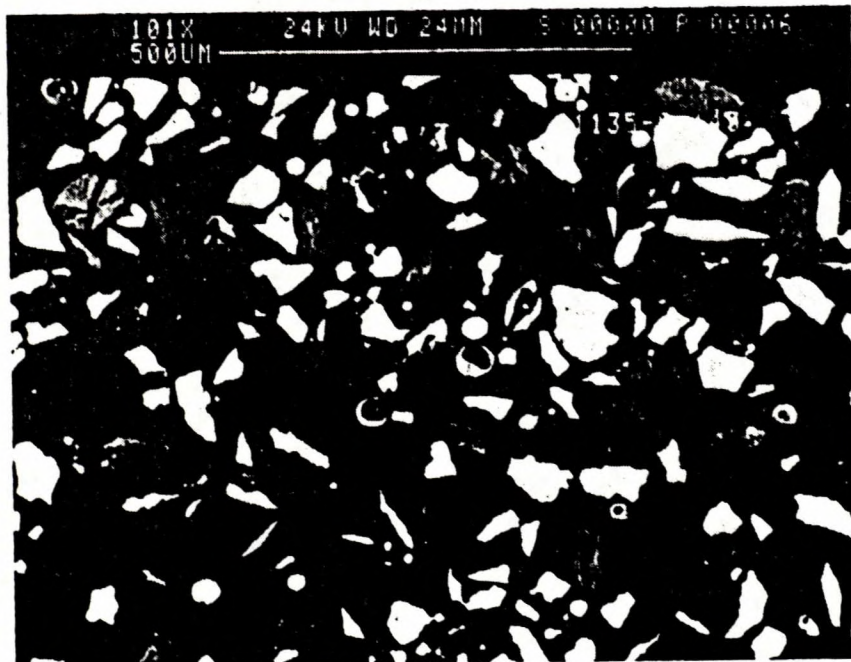
Figure 12 - S.E.M. photo of combusted residue from Geco 1135
