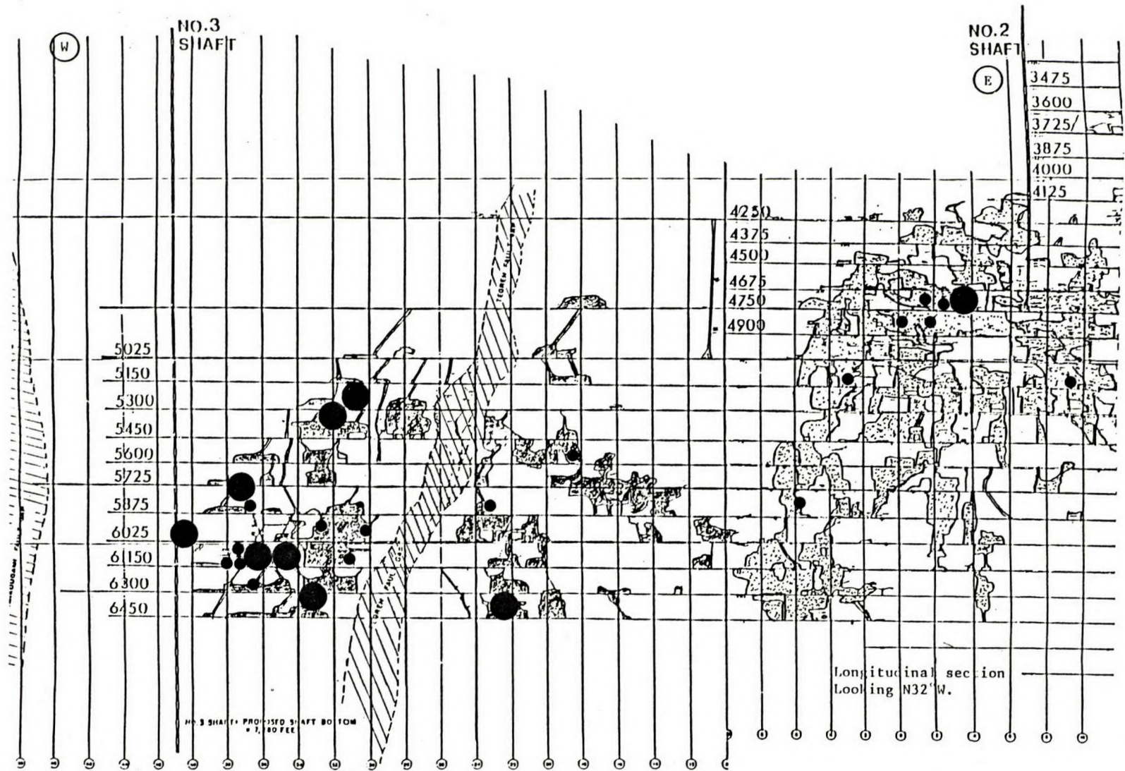
Fig. 3 - Location of rockbursts on the west and central area at the Macassa Mine. (●) Recorded rockbursts, magnitude 2.2 to 3.1 MN. (●) observed "heavy rockbursts", rock displacement >50 tons.
