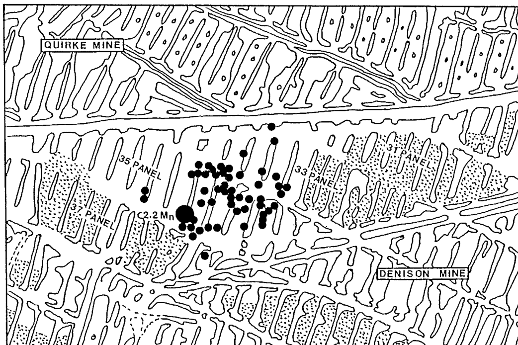
Fig. 2 - Locations of seismic events at Denison Mine during May, 1986.
