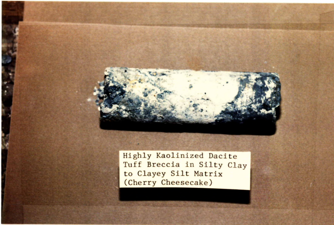
Figure 17. Core recovery using improved techniques: very weak, highly kaolonized dacitic tuff breccia in a silty clay to clayey silt matrix "cherry cheesecake" (4).
