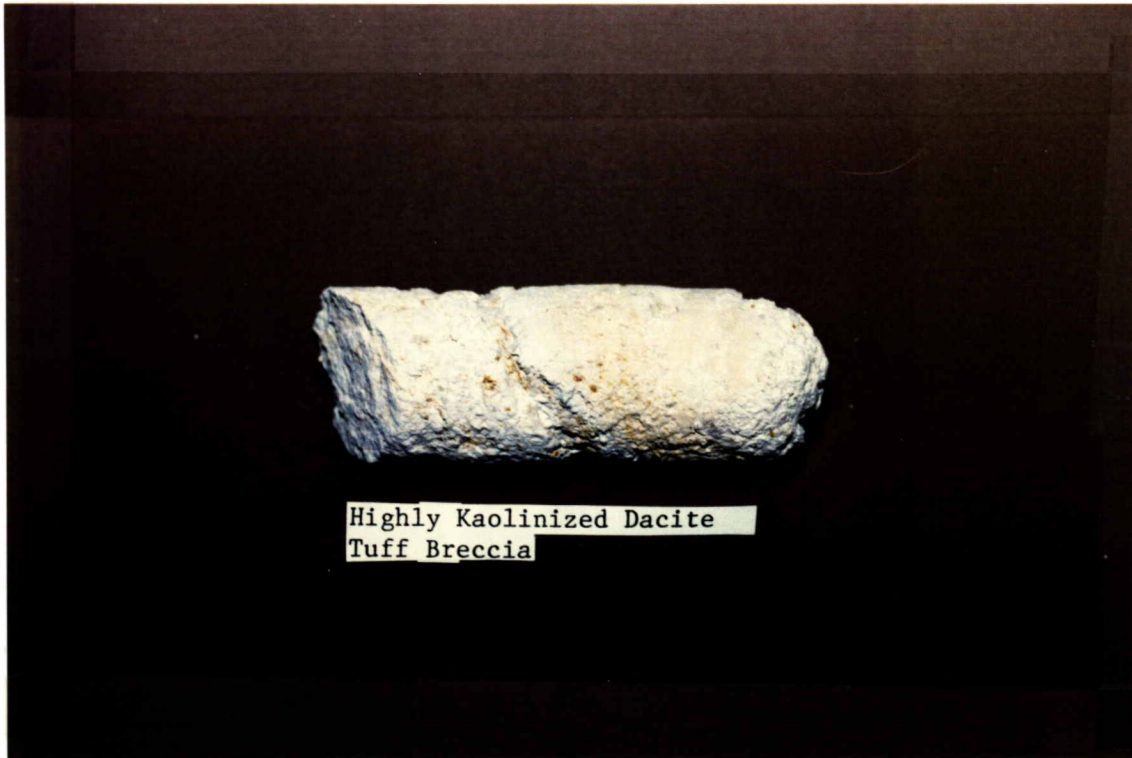
Figure 16. Core recovery using improved techniques: very weak, highly kaolinized dacitic tuff breccia (4).
