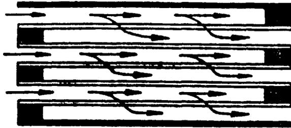
Figure 2 - Ceramic Element Soot Filtration Principle
