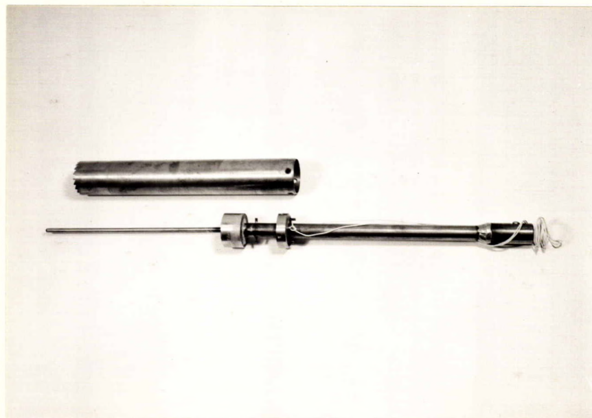
GROUTING TOOL DISMANTLED.
