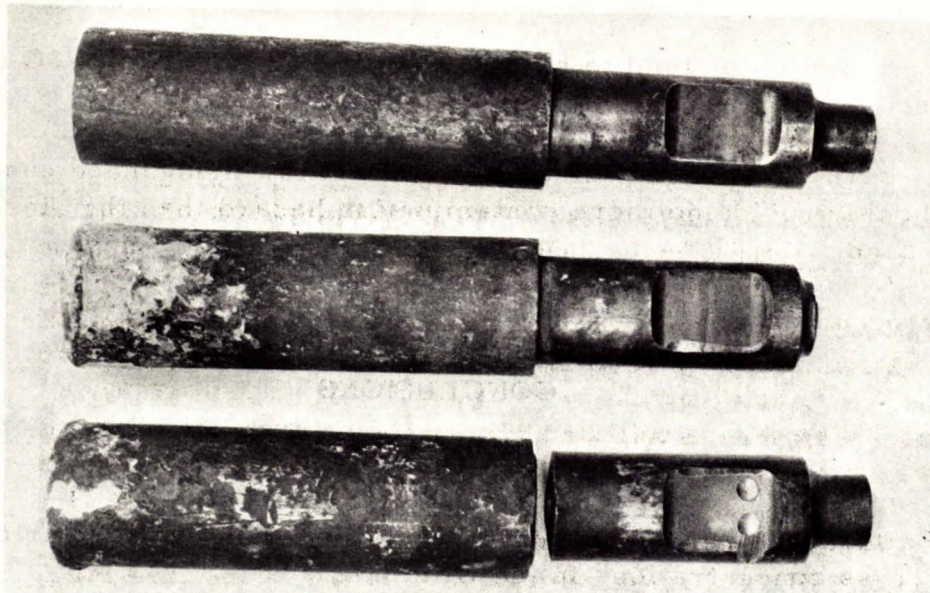
Figure 1. Crust breaking tools showing two broken at fillets and one unused fillet. As Received, X1/4.
