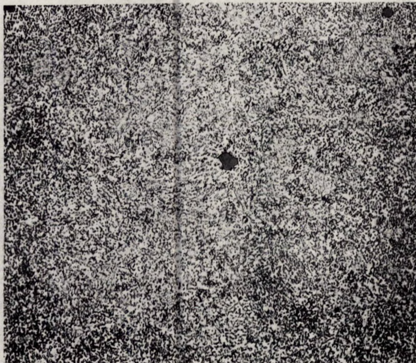
Figure 4. Photomicrograph of a section through the cutting edge of the blade, showing sulphide inclusions.
