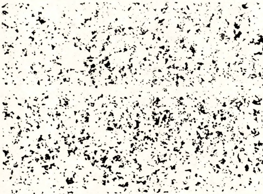
Figure 1. "Nickel Silver" Alloy. Transverse section showing general porosity.
