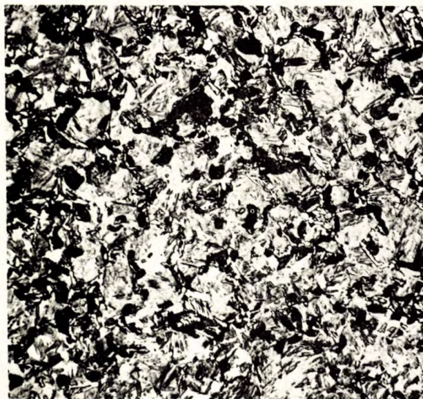
(RC46) X500 2% nital etch (a)
