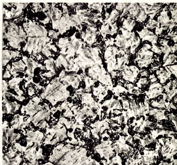
(RC50) X500 2% nital etch (b)
