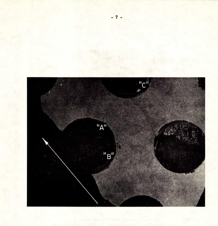
Figure 2. Macrophotograph showing corrosion pits and dense adherent deposits in the suction roll holes. The main fracture cuts across the lower left part of the field in the direction of the arrow. Small cracks are visible at locations "A", "B" and "C". Etched in Vilella's reagent. (X9)
