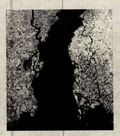
Figure 3. Crack radiating from corrosion pits at location "A" in Figure 2. This crack started in the direction of inclusion stringers and then turned 90 degrees to the left to parallel the main fracture. Etched in Vilella's reagent. (X500)
