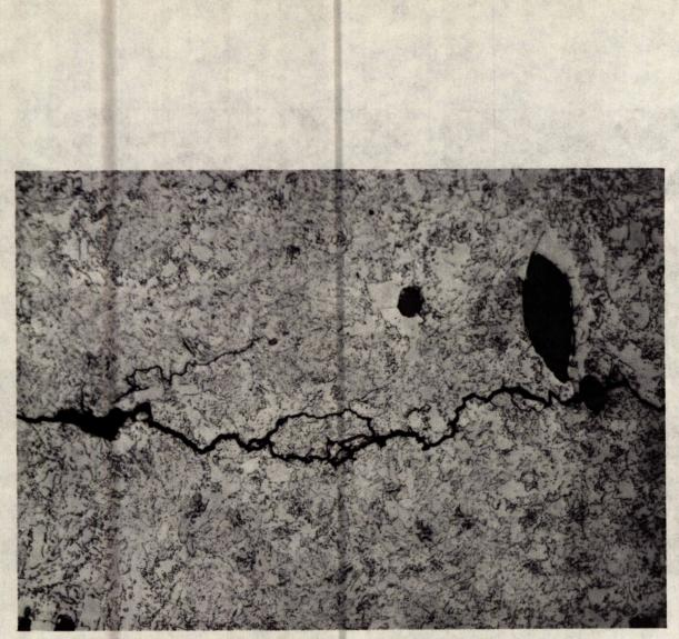
Figure 5. Photomicrograph of cracked region. "C". This is a representative field, where the path of the crack has not been obscured by corrosion, showing that the cracks progressed intergranularly without many secondary cracks. Et ched in Vilella's reagent. (X500)
