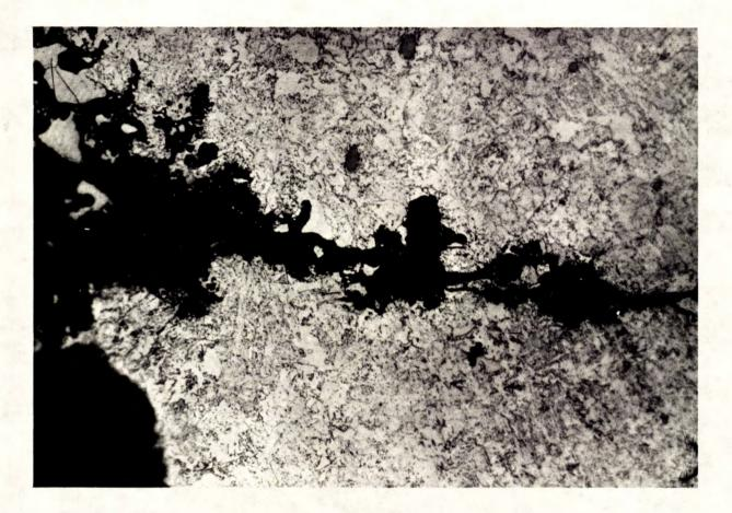
Figure 4. Crack radiating from corrosion pits at location "B" in Figure 2. The path of this crack is directly across the longitudinal forging direction. Pitting and general corrosion attack within the crack is evident. Etched in Vilella's reagent. (X500).
