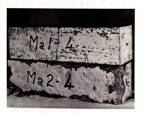
Figure 1 - Series A: Medium Strength Concrete Mixes 1 and 2 After 32 Freeze-Thaw Cycles
