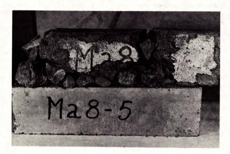
Figure 3 - Series B: Low Strength Concrete Mixes 5 and 8 After freeze-thaw cycling
