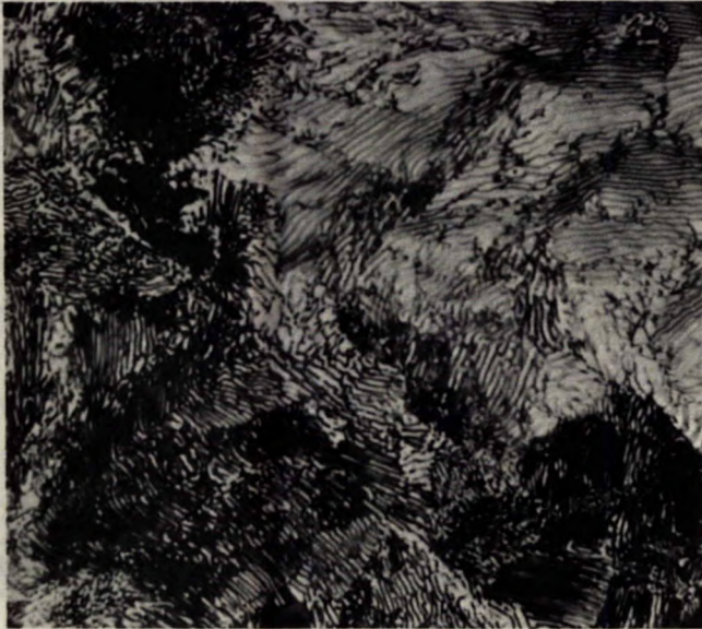
Quebec Cartier, Rlwy. USS Standard Carbon Steel Rail - \frac{1}{4} in. from crown head surface
