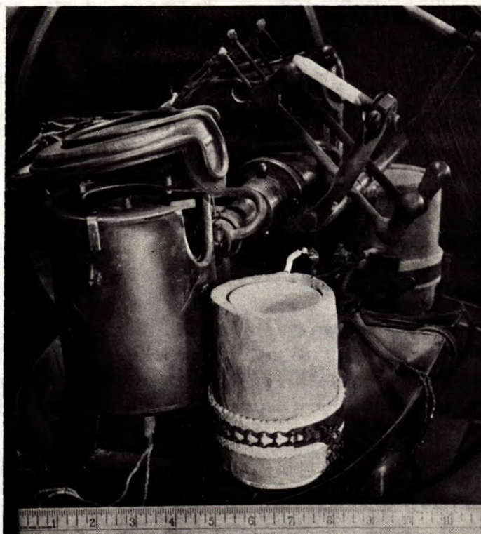
Figure 1. Vacuum melting furnace.
