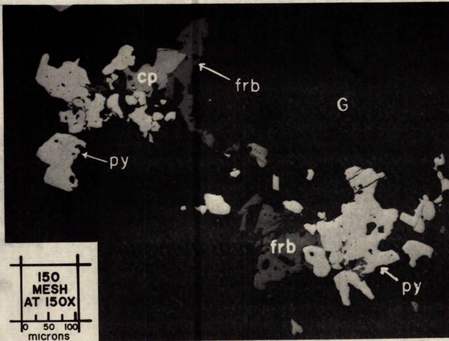
Figure 2. Photomicrograph of a polished section of the ore showing a field that contains pyrite (py), chalcopyrite (cp), freibergite (frb) and gangue (G).
