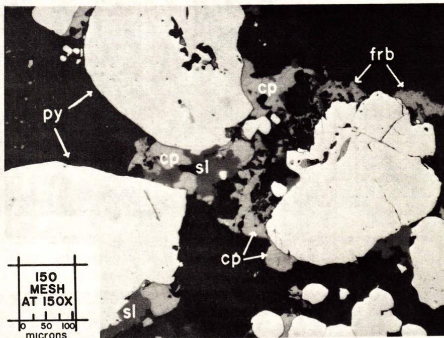
Figure 1. Photomicrograph of a polished section of the ore showing a field that contains pyrite (py), chalcopyrite (cp), sphalerite (sl) and freibergite (frb). The dark background represents gangue.
