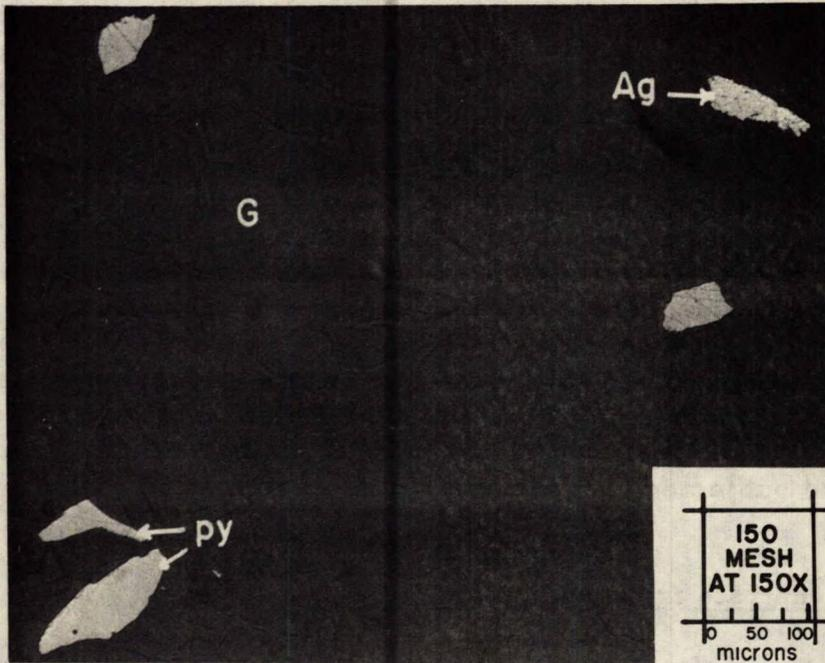
Figure 4. Photomicrograph of the flotation tailing concentrate showing one grain of native silver (Ag) and a few grains of pyrite (Py) with a large number of grains of gangue (G).
