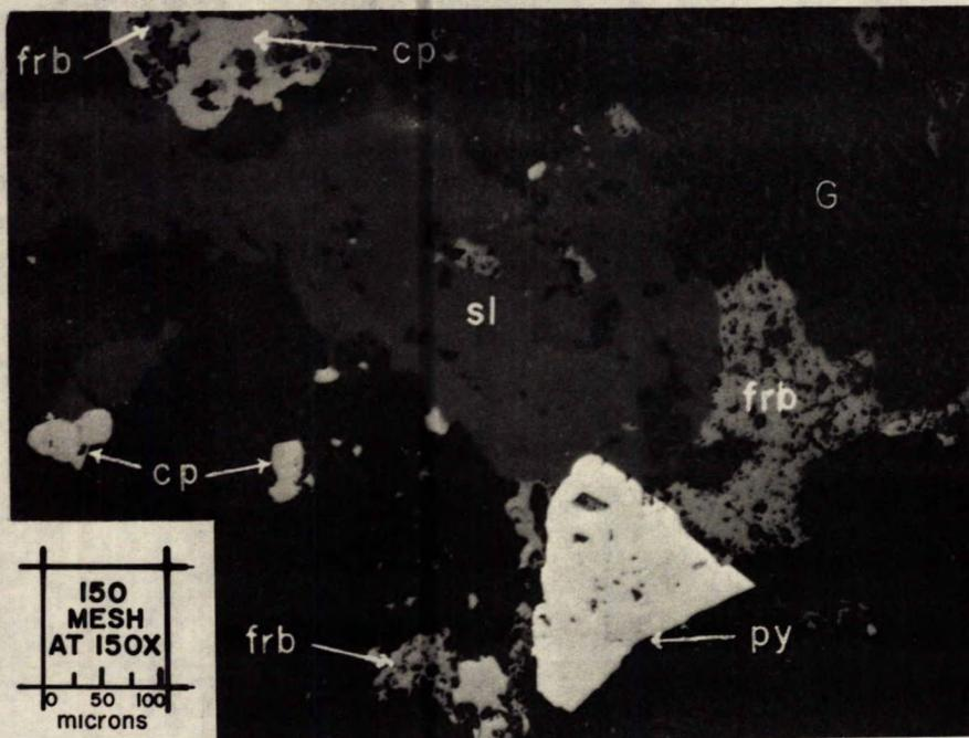
Figure 3. Photomicrographs of a polished section of the ore showing a field that contains sphalerite (sl), freibergite (frb), chalcopyrite (cp), pyrite (py) and gangue (G).
