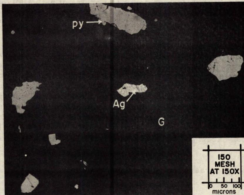
Figure 5. Photomicrograph of the cyanidation residue concentrate showing one grain of native silver (Ag) a few grains of pyrite (Py) and gangue (G).
