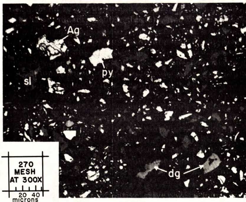
Figure 2. Photomicrograph of the May 12 lead rougher concentrate. The principal minerals shown are pyrite (py) and sphalerite (sl), a few of which are labelled. One combined grain of native silver (Ag) and pyrite is shown. Several grains of digenite (dg) are present.
