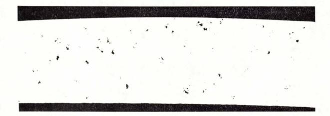
Figure 1 - Section through cover showing microporosity. (Unetched).
