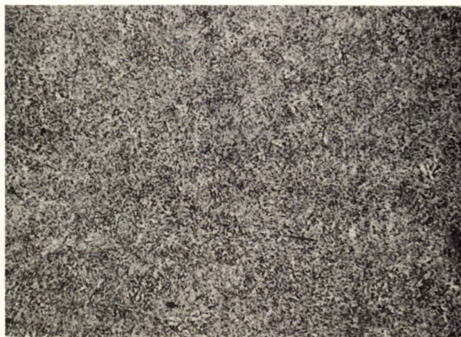
Figure 11. Sample No.3. Reheat treated as in Figure 9 (R C 50). Charpy V-notch fractures were much finer grained than those observed in the as-received springs.
