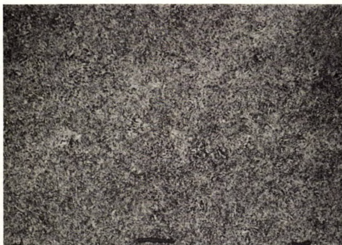
Figure 10. Sample No.2. Reheat treated as in Figure 9. (R C 50). The banded structure and grain boundary constituent appear to have been eliminated.
