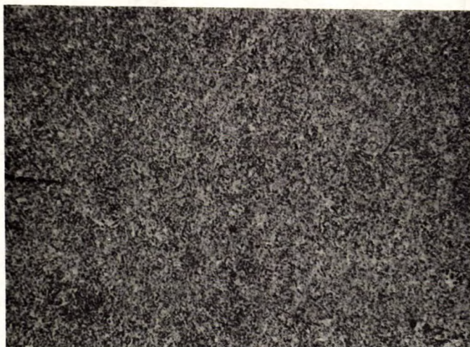
Figure 9. Sample No.1. Reheat treated; normalized 1650°F (1 hr); oil quenched from 1550°F. Tempered 700°F; water quenched - R C 50. Shepherd grain size is No.8. The banding is eliminated or masked. No trace of grain boundary constituent was observed.
