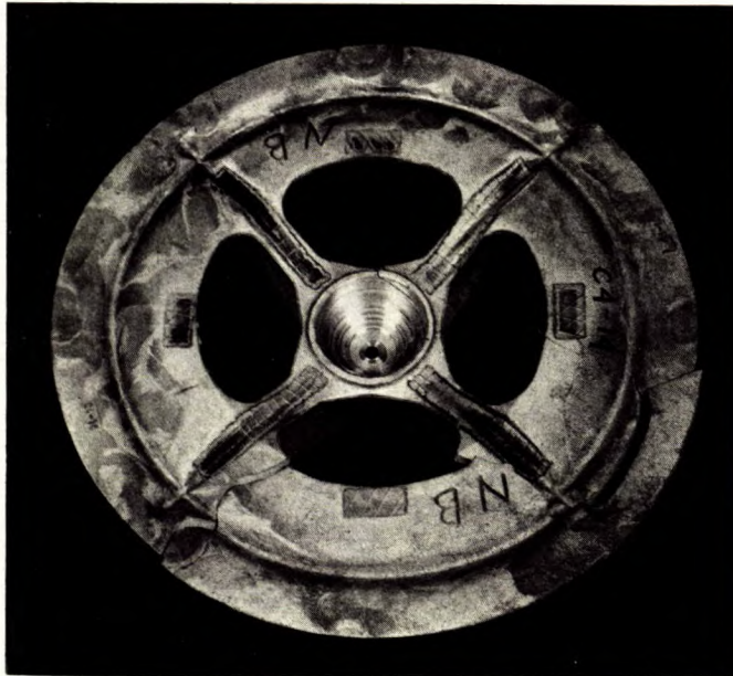
Figure 15. Fracture of casting of C4 design due to unsoundness in reinforcing rib (tested in sand).
