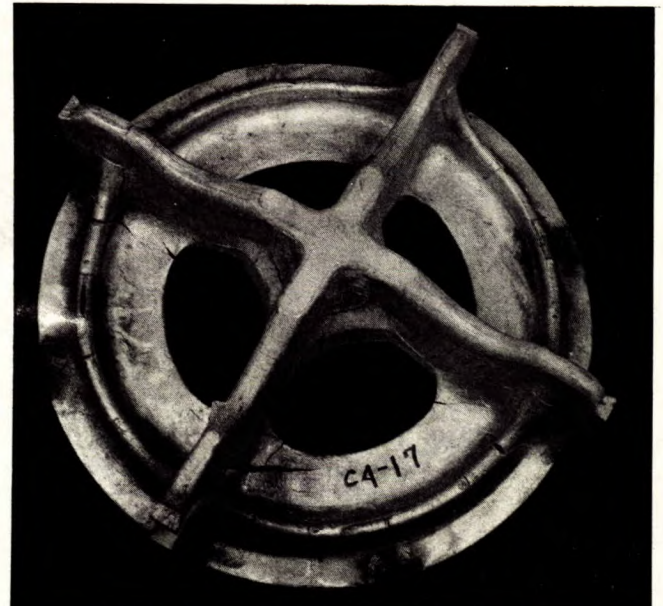
Figure 16. Mode of fracture with satisfactory soundness in both the socket area and the reinforcing rib.
