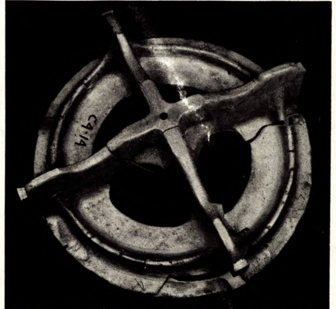
Figure 15. Fracture of casting of C4 design due to unsoundness in reinforcing rib (tested in sand).
