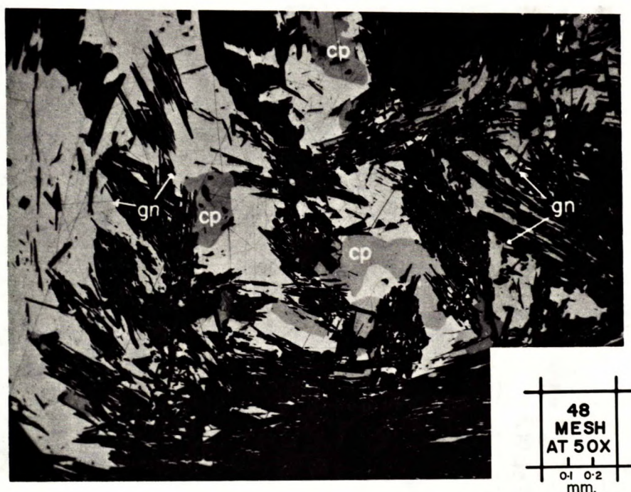
Figure 2. Photomicrograph of a polished section of Sample 25 showing galena (gn) and chalcopyrite (cp) in gangue (black).
