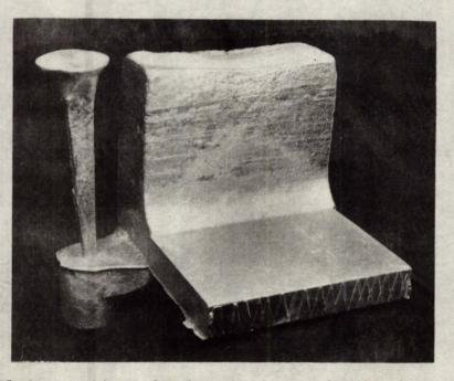
Figure 2. Plate casting showing gating and risering. The chilled face can be seen in the foreground.
