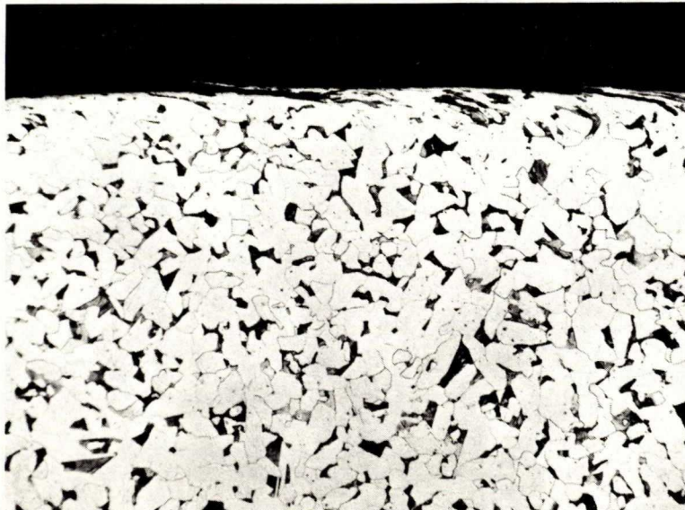
Figure 2. (a) Unworn surface not carburized (b) Worn surface showing worked metal.
