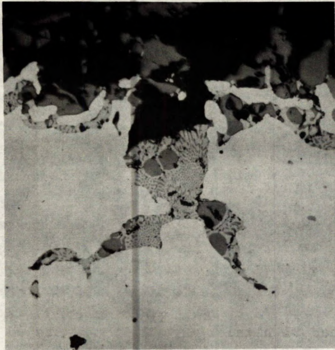
Figure 8. Corrosive Attack by Fused Sulphur-rich Slag at Outside Surface. The eutectic phase was identified as \text{FeO.FeS} and has a melting point of approximately 1000^{\circ}\text{C} ( 1832^{\circ}\text{F} ).
