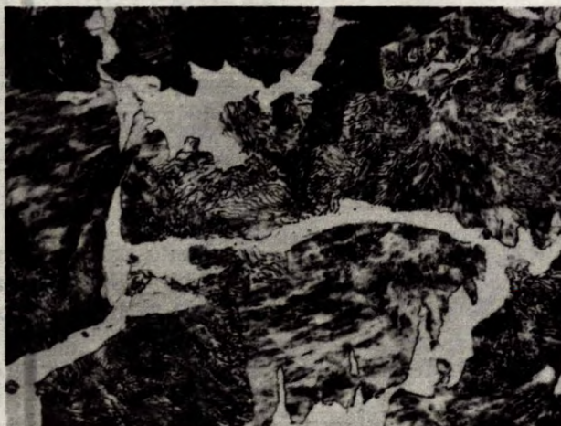
Base Metal (as-rolled or normalized structure)
