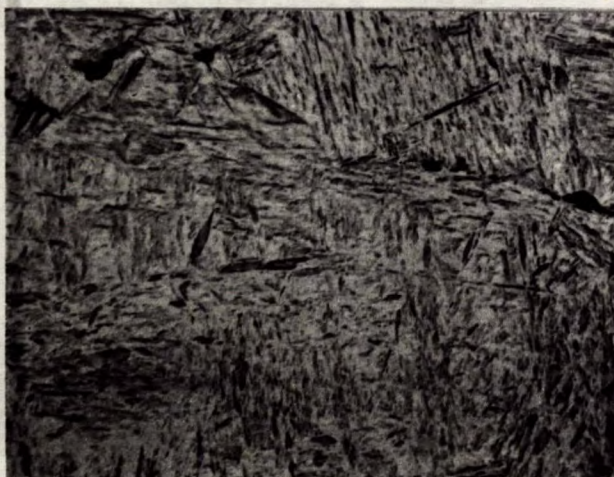
Martensite in Base Metal (underlying the weld deposit)
