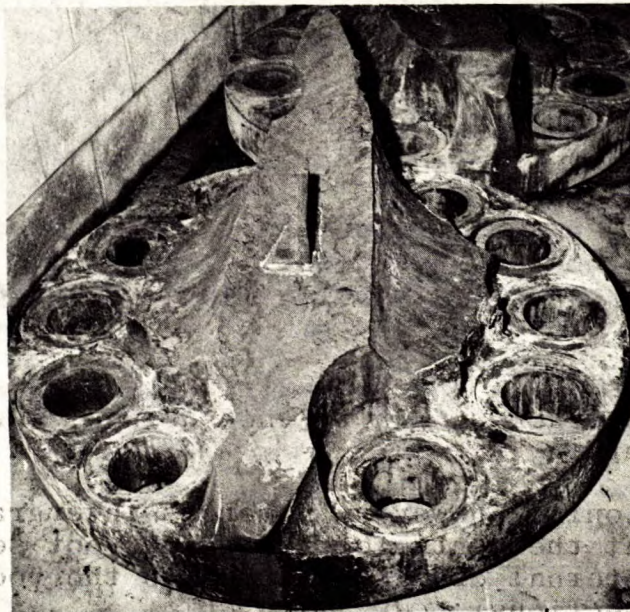
Figure 2. Broken Blade, CCGS John A. MacDonald, Sample "R" (3 views). The fracture is brittle and shows little evidence of plastic deformation. The fracture surface is more irregular than that illustrated in Figure 1.
