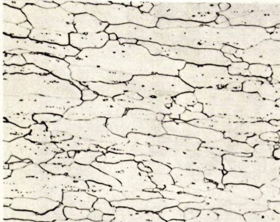
Figure 5. Microstructure of fin steel from A-end of Sample 1. Nital etch, X500.
