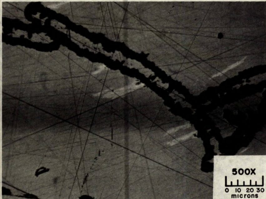
Figure 3 - Photomicrograph of a polished section showing minute elongated inclusions of pentlandite (white) in pyrrhotite (grey). The black areas are pits on the polished surface.
