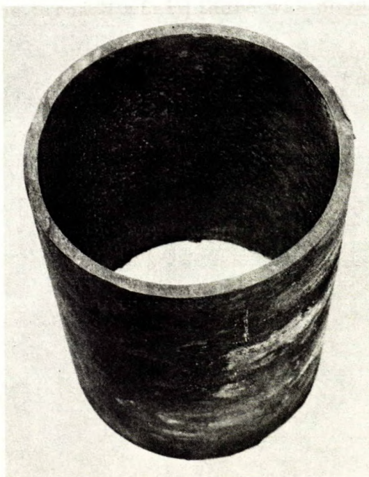
Figure 2. Sample A. Illustrates exposed surface of tube and slag coating. Droplets of slag are shown, (arrow 1). The appearance of the tube surface after removal of the slag is shown, (arrow 2).
