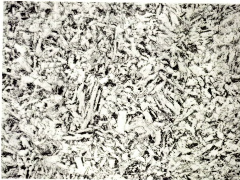
Figure 5. CF-IGG Starboard Front. Etched in 2% nitric acid in alcohol. X500.
