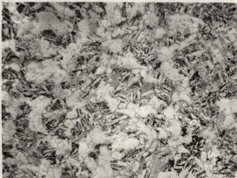
Figure 6. CF-OBN Starboard Front. Etched in 2% nitric acid in alcohol. X500.
