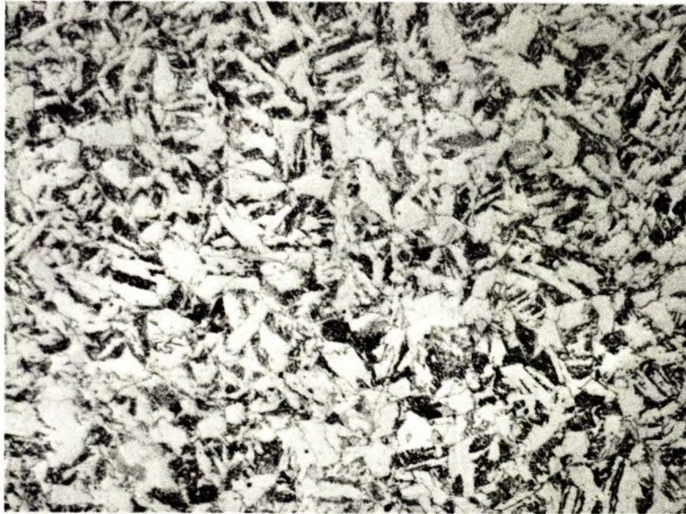
Figure 4. CF-BHW Port Rear. Etched in 2% nitric acid in alcohol. X500.
