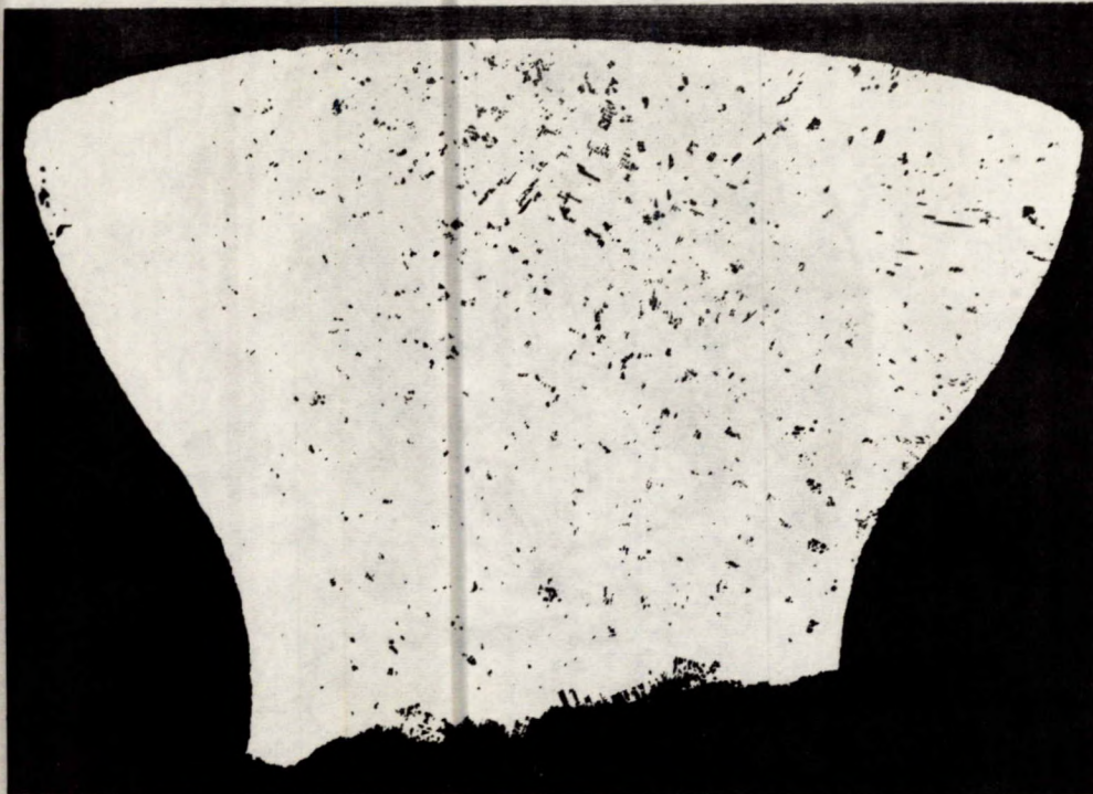
Figure 3. Other half of bolt from Figure 2 after polishing shows very severe general porosity.
