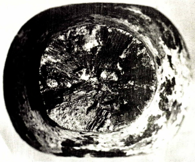
Figure 1. Fracture showing oxidized area (right), presumably the site of an old crack, and dendrites.
