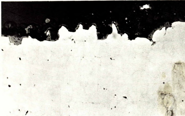
Figure 6 X150 Section through the fracture of the broken anchor bolt. The presence of an oxide layer on part of the fracture indicates that a crack had taken place sometime before the final failure. As-polished.
