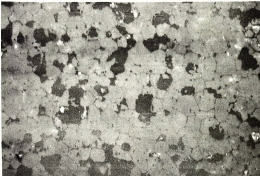
(b) Group C. Disk made from uncalcined precipitate 17-62. Forming pressure 5.6 \times 10^3 kg/cm 2 . Sintered at 1225°C for 30 minutes.
