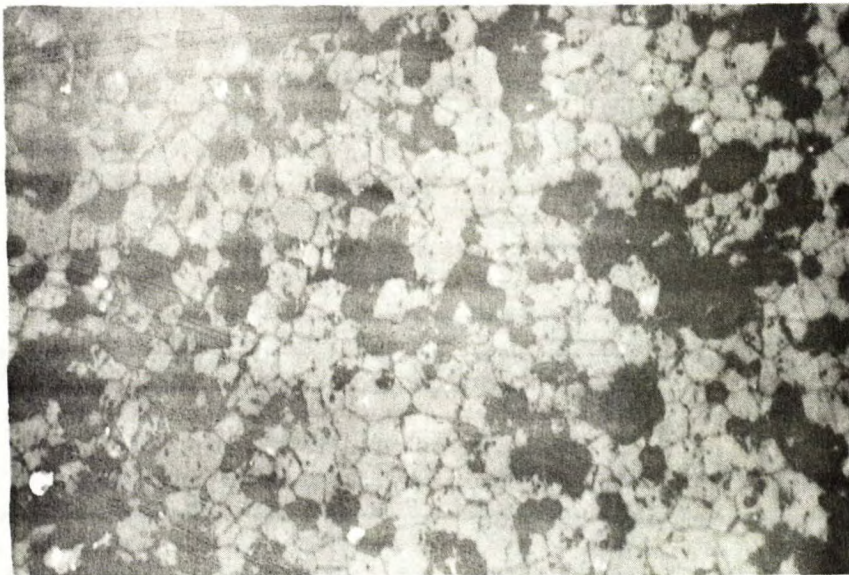
(a) Group A. Disk made from uncalcined precipitate 17-57 and sintered at 1225°C for 60 minutes. Forming pressure 2.8 \times 10^3 kg/cm 2 .
