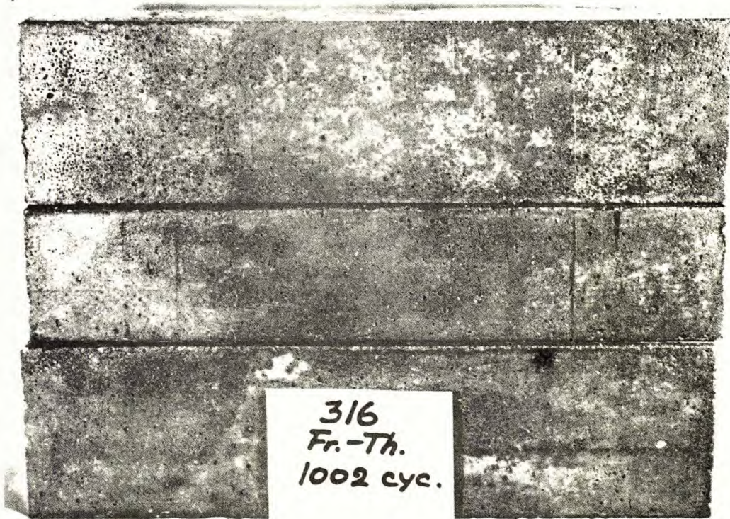
Figure 1. Series B-280 containing Darex and WRDA; concrete specimens show slight surface scaling after 1002 freeze-thaw cycles.
