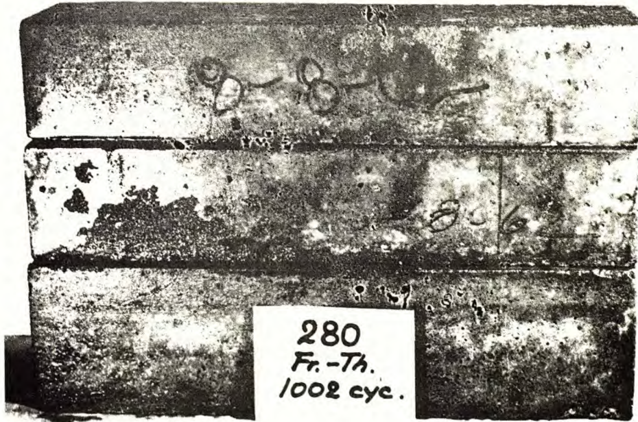
Figure 1. Series B-280 containing Darex and WRDA; concrete specimens show slight surface scaling after 1002 freeze-thaw cycles.
