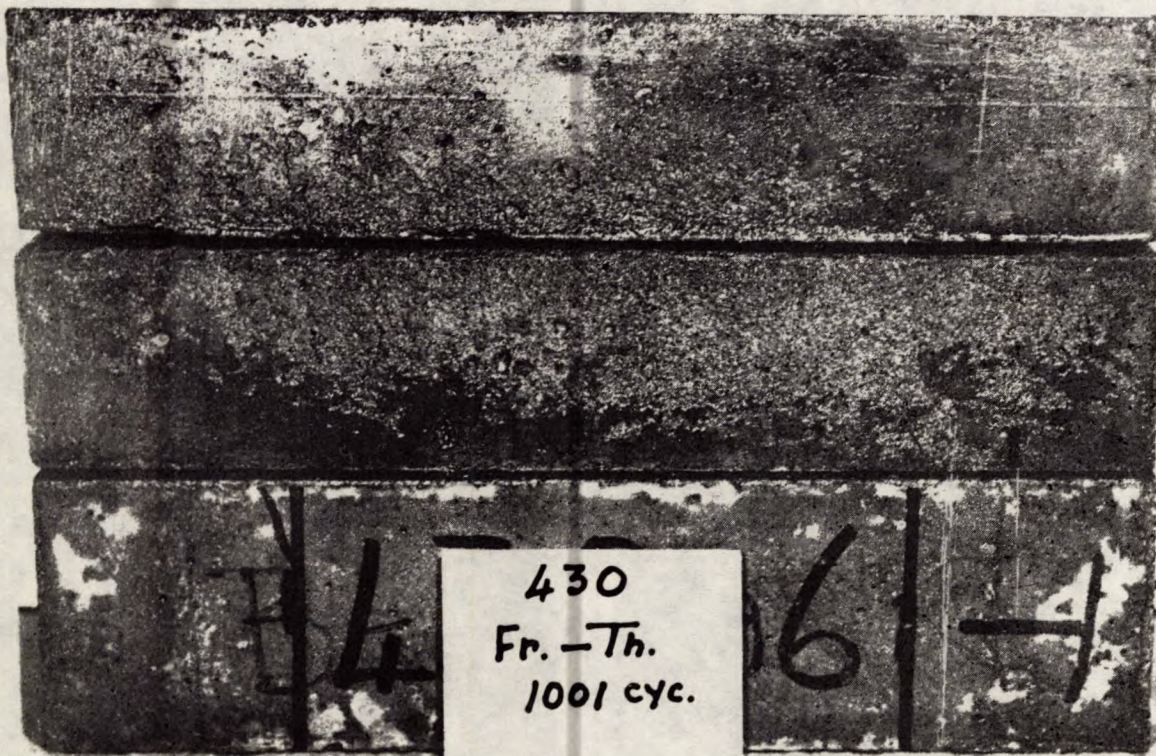
Figure 4. Series B-430 containing MBVR and Pozzolith shows slight surface scaling after 1001 freeze-thaw cycles.
