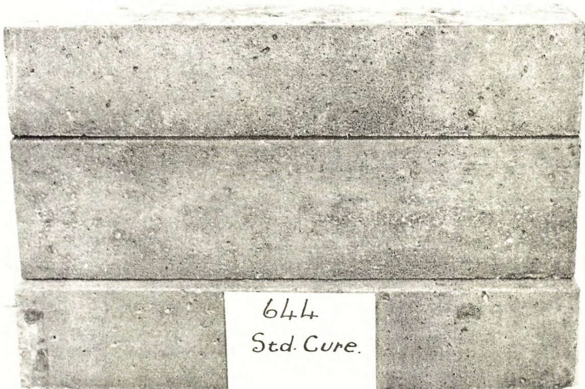
Figure 8b. Series B-644 containing Darex AEA; reference test specimens.
