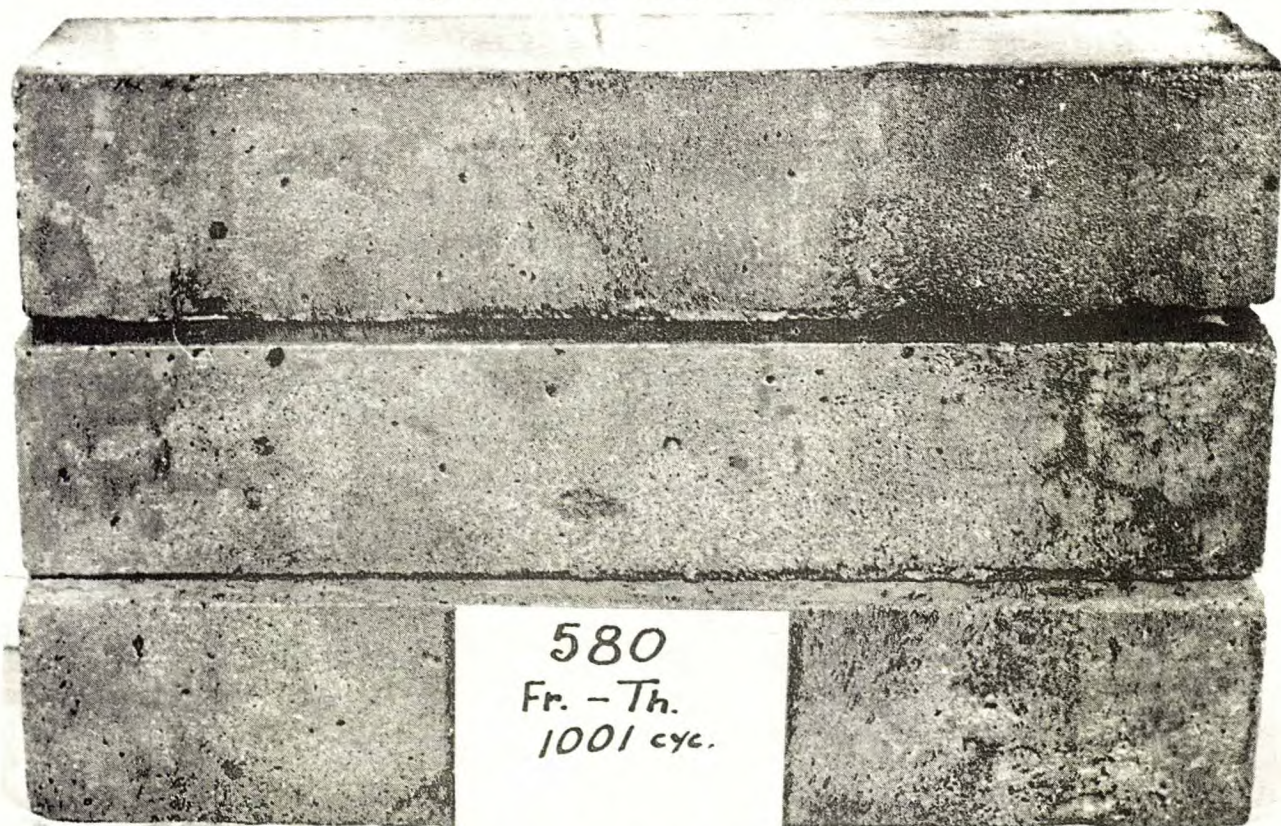
Figure 6. Series B-580 containing Cyrigel shows no signs of deterioration after 1001 freeze-thaw cycles.
